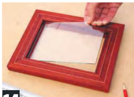
14 Cut 2mm glass to size or order this from a glazier. A piece of 3mm hardboard or MDF is ideal for backing
